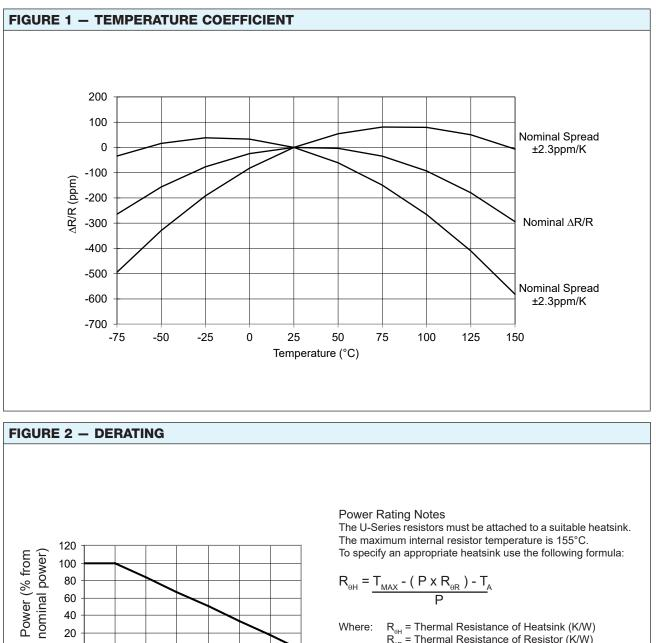
$R_{_{\Theta H}} = \text{Thermal Resistance of Heatsink (K/W)} \\ R_{_{\Theta R}} = \text{Thermal Resistance of Resistor (K/W)} \\ T_{_{MAX}} = \text{Maximum Temperature of Resistor} \\ T_{_{A}} = \text{Ambient Temperature of Heatsink (°C)}$ Where: P = Power Through Resistor (W)
